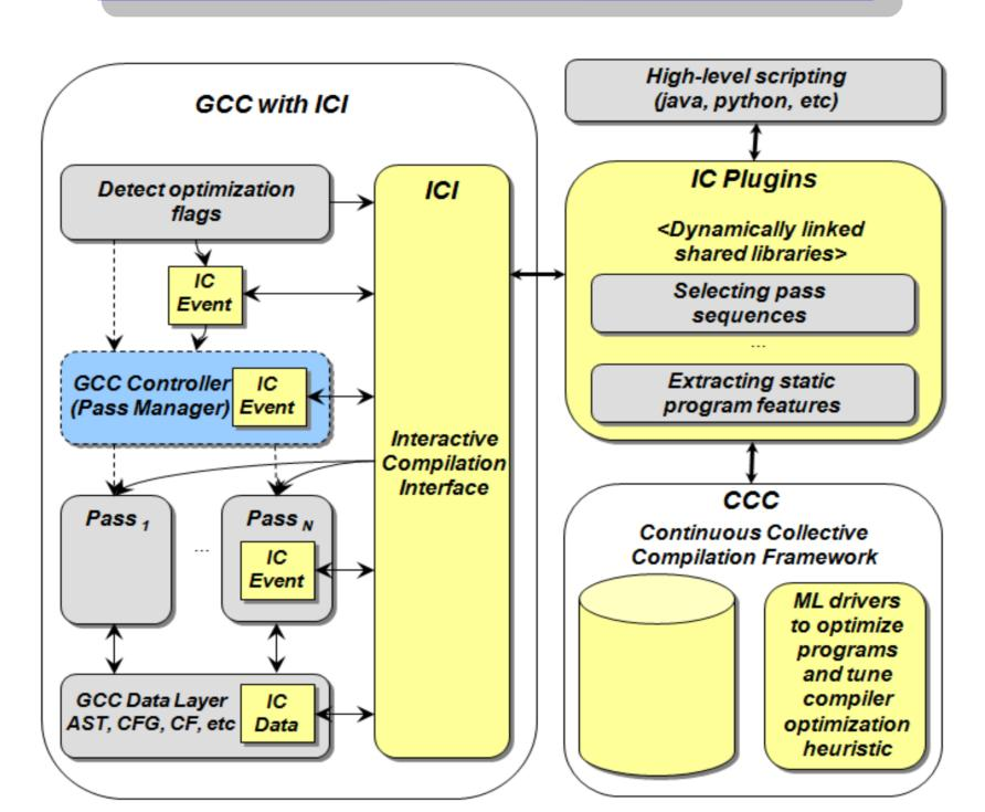
The ICI provides opportunities for external control and examination of the compiler. Optimization settings at a fine-grained level, beyond the capabilities of command line options or pragmas, can be managed through IC plugins.
