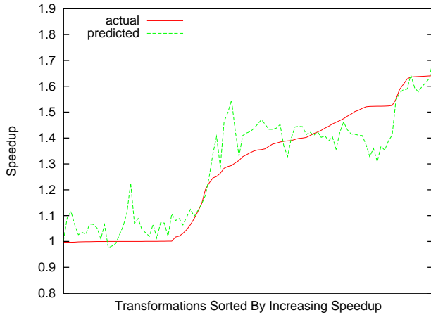
Figure 1: Model accuracy for compress . The y-axis corresponds to the speedup of each transformation sequence relative to the original untransformed program. The x-axis corresponds to transformation sequences sorted in increasing order of performance. The line marked actual corresponds to the real measured performance of the program while predicted corresponds to the prediction of our model. The prediction is averaged over 30 trials.
