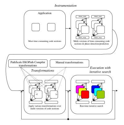
Fig. 2. Application instrumentation and multi-versioning for run-time iterative optimization
