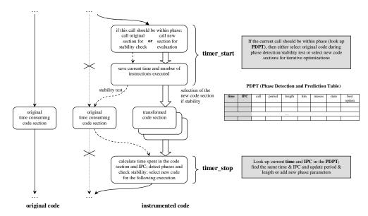
Fig. 7. Code instrumentation for run-time adaptive iterative optimizations.
