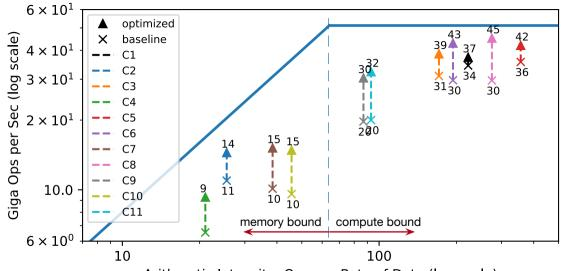
Arithmetic Intensity: Ops per Byte of Data (log scale)
